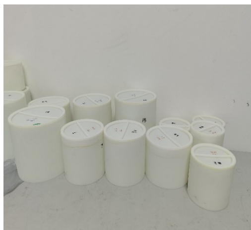
图2 3D打印样品盒设计图及实物图 Fig.2 Design and physical drawing of 3D printing Marinelli beakers
